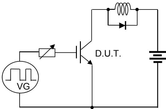
Fig.18 Inductive Load Circuit
