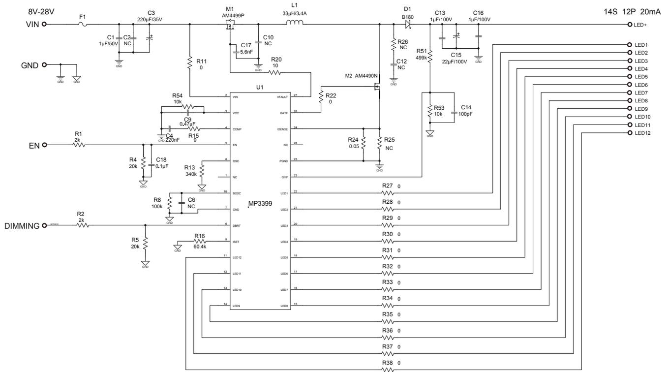
Figure 6—Drive 14 LEDs in Series, 12 Strings 20mA/string
