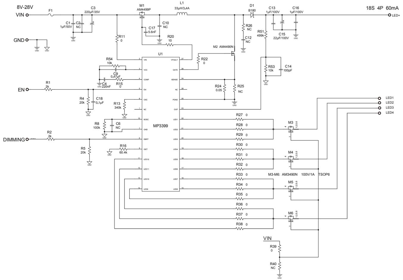
**Figure 8 – Drive 18LEDs in Series, 4 strings 60mA/string**
