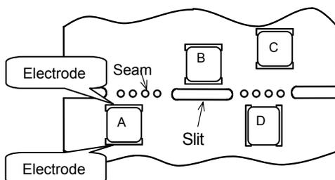
\*1 A > D is valid when stress is added vertically to the perforation as with Hand Separation. If a Cutting Disc is used, stress will be diagonal to the PCB, therefore A > D is invalid.
