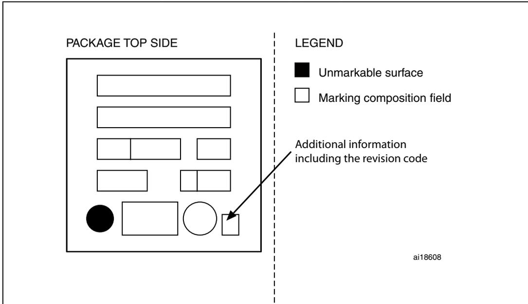
Figure 2. LQFP48 and LQFP32 top package view
