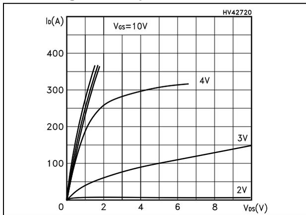
Figure 5. Transfer characteristics
