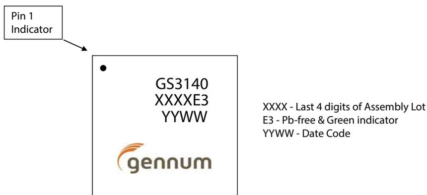
Figure 7-3: Marking Diagram
