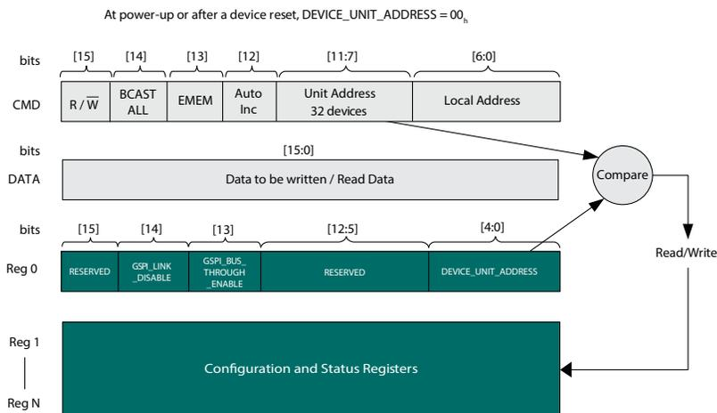
**Figure 4-18: Internal Register Map Functional Block Diagram**
