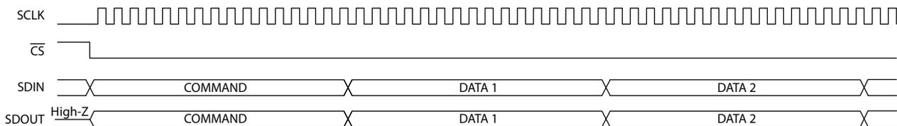
**Figure 4-15: GSPI Write Timing – Auto-Increment with Bus-Through Operation**
