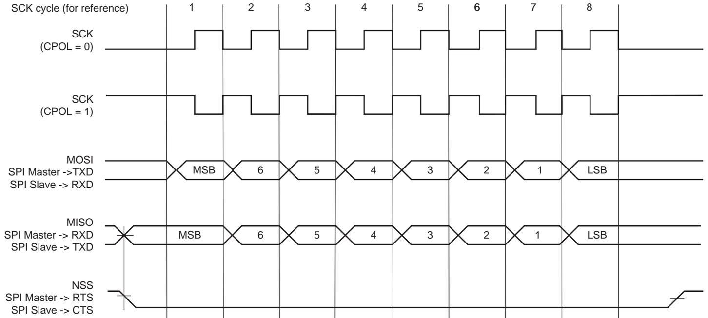
**Figure 33-24. SPI Transfer Format (CPHA = 0, 8 bits per transfer)**
