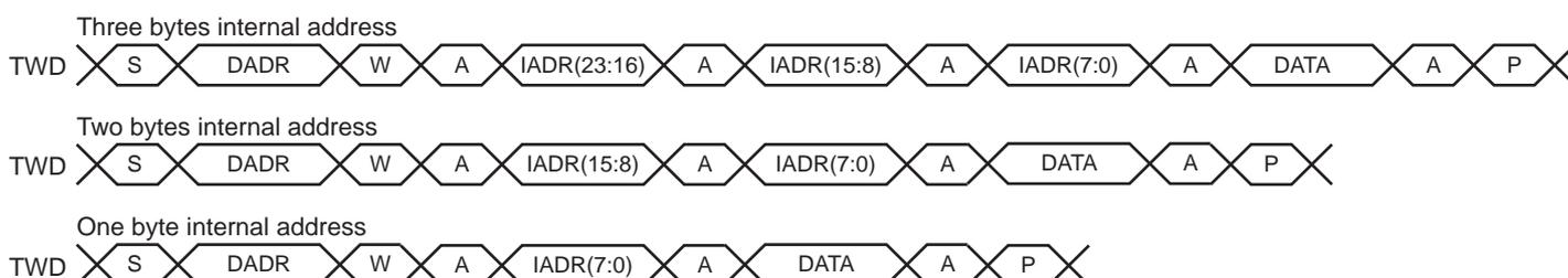
**Figure 29-12. Master Read with One, Two or Three Bytes Internal Address and One Data Byte**
