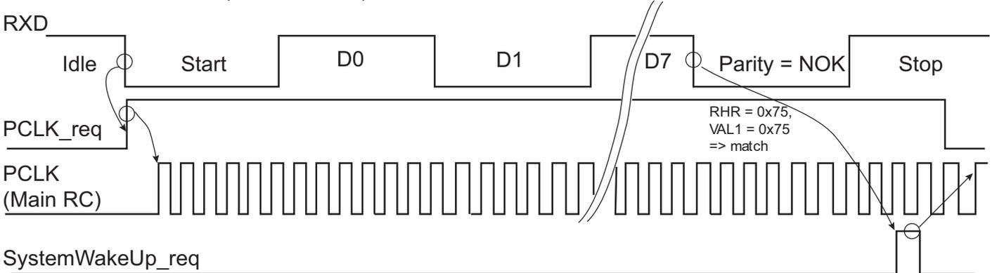
**Figure 32-13. Asynchronous Event Generating Only Partial Wake-up**
