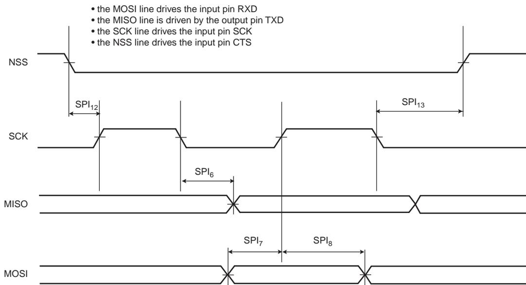
**Figure 36-17. USART SPI Slave Mode (Mode 0 or 3)**
