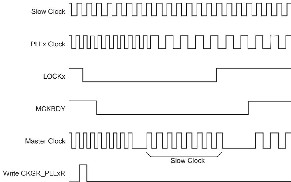
**Figure 24-10. Programmable Clock Output Programming**
