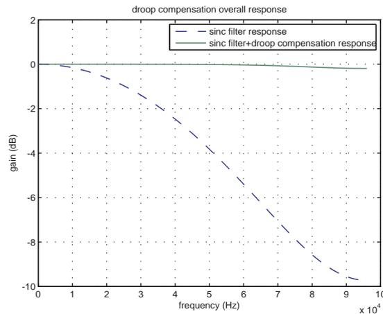
**Figure 31-6. Droop Compensation Filter 0 to 20 kHz Band Flatness**
