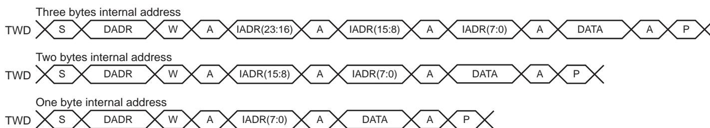
**Figure 28-14. Master Read with One, Two or Three Bytes Internal Address and One Data Byte**
