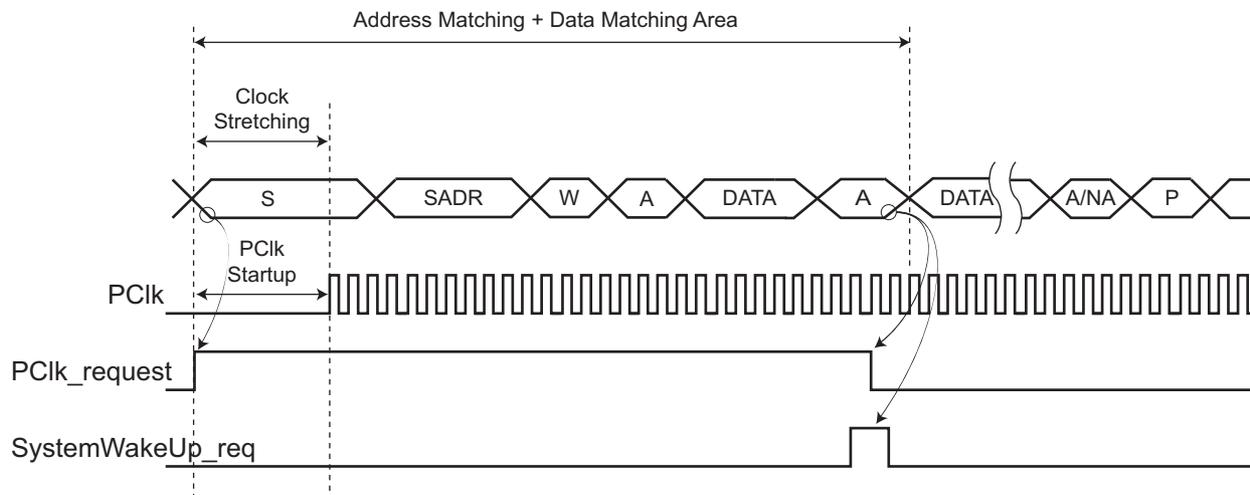
**Figure 28-47. Address Match and No Data Match (Data Matching Enabled)**
