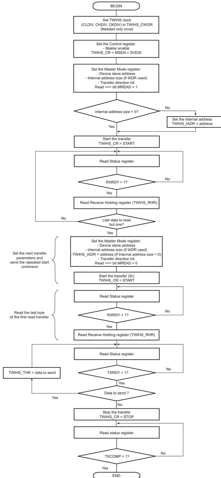
Figure 28-30. TWIHS Read Operation with Multiple Data Bytes + Write with Alternative Command Mode with PEC
