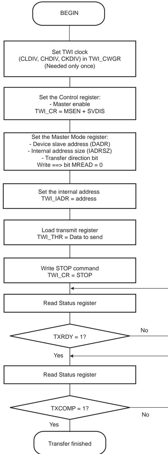
Figure 29-17. TWI Write Operation with Multiple Data Bytes with or without Internal Address
