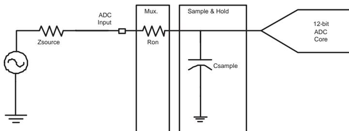
During the tracking phase, the ADC must track the input signal during the tracking time shown below:
