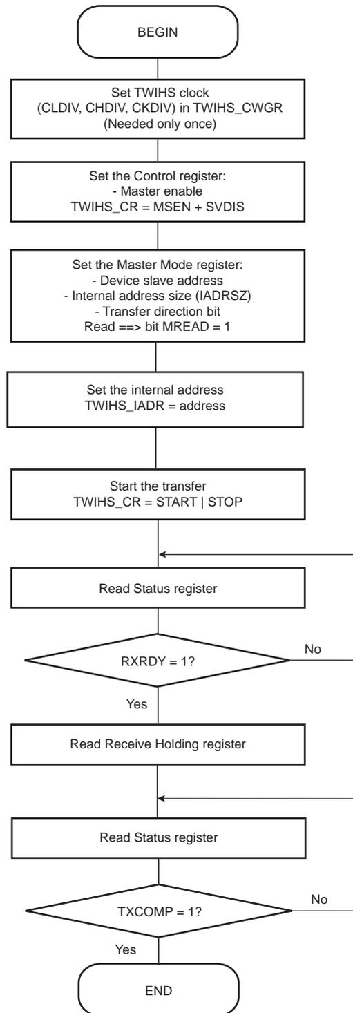
Figure 28-26. TWIHS Read Operation with Multiple Data Bytes with or without Internal Address
