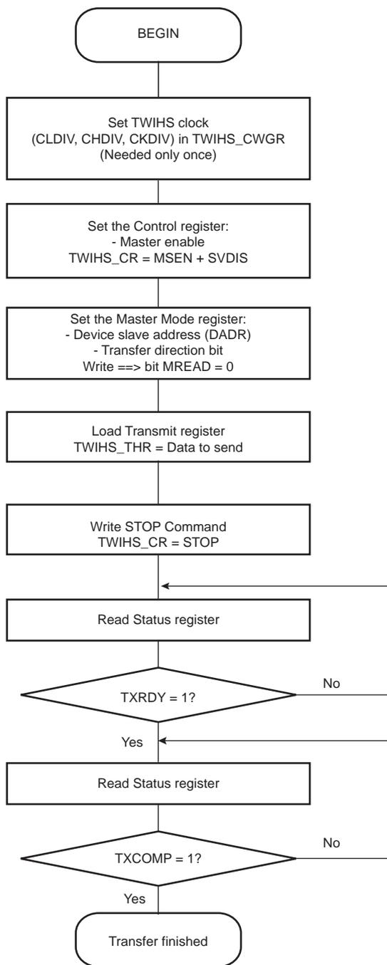
**Figure 28-18. TWIHS Write Operation with Single Data Byte and Internal Address**
