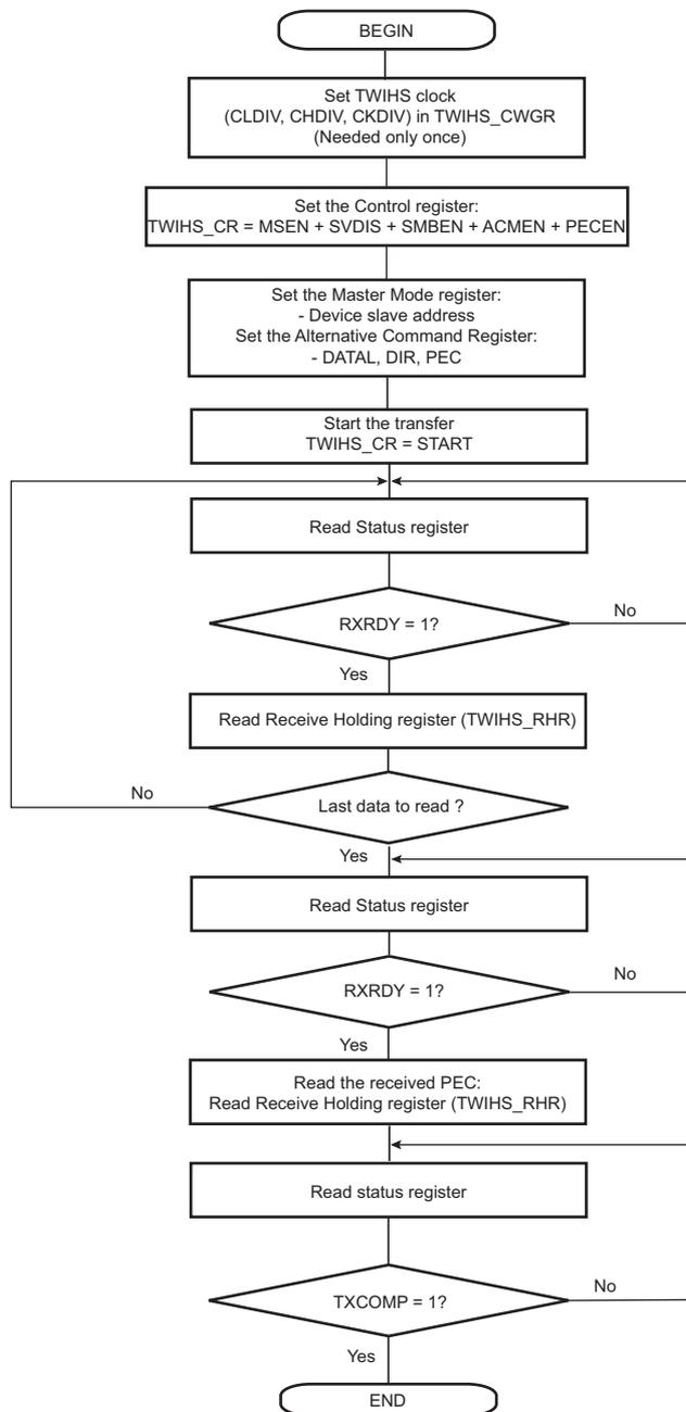
Figure 28-29. TWIHS Read Operation with Multiple Data Bytes + Write Operation with Multiple Data Bytes (Sr)
