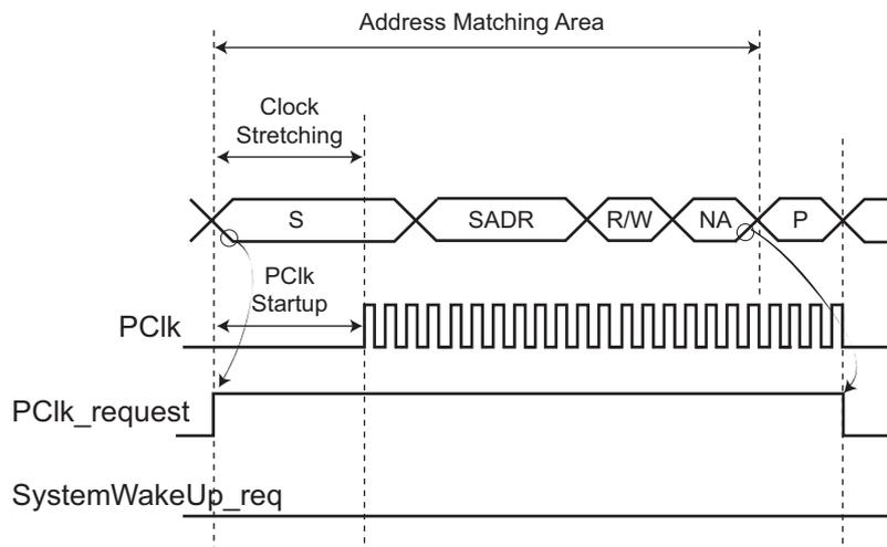
**Figure 28-46. Address Match and Data Match (Data Matching Enabled)**
