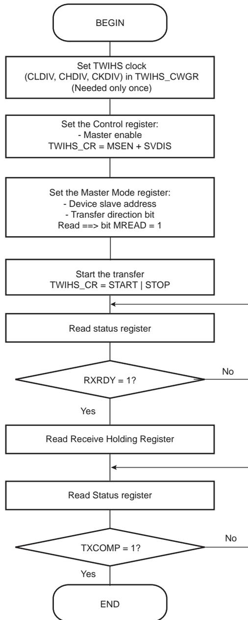
Figure 28-25. TWIHS Read Operation with Single Data Byte and Internal Address
