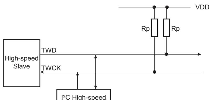
Figure 28-35. Fast Mode Slave Mode Typical Application Block Diagram
