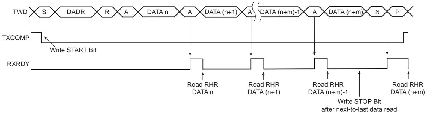
**Figure 28-12. Master Read Clock Stretching with Multiple Data Bytes**
