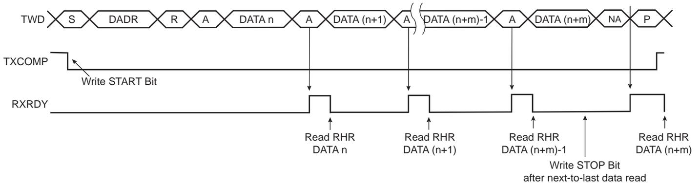
**Figure 29-10. Master Read Wait State with Multiple Data Bytes**
