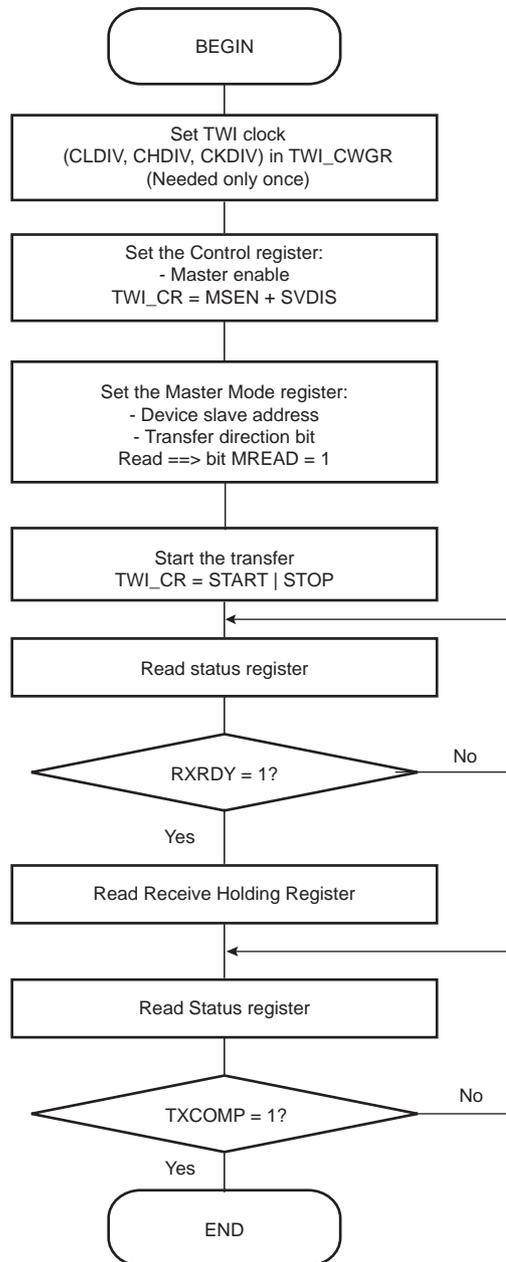
**Figure 29-19. TWI Read Operation with Single Data Byte and Internal Address**
