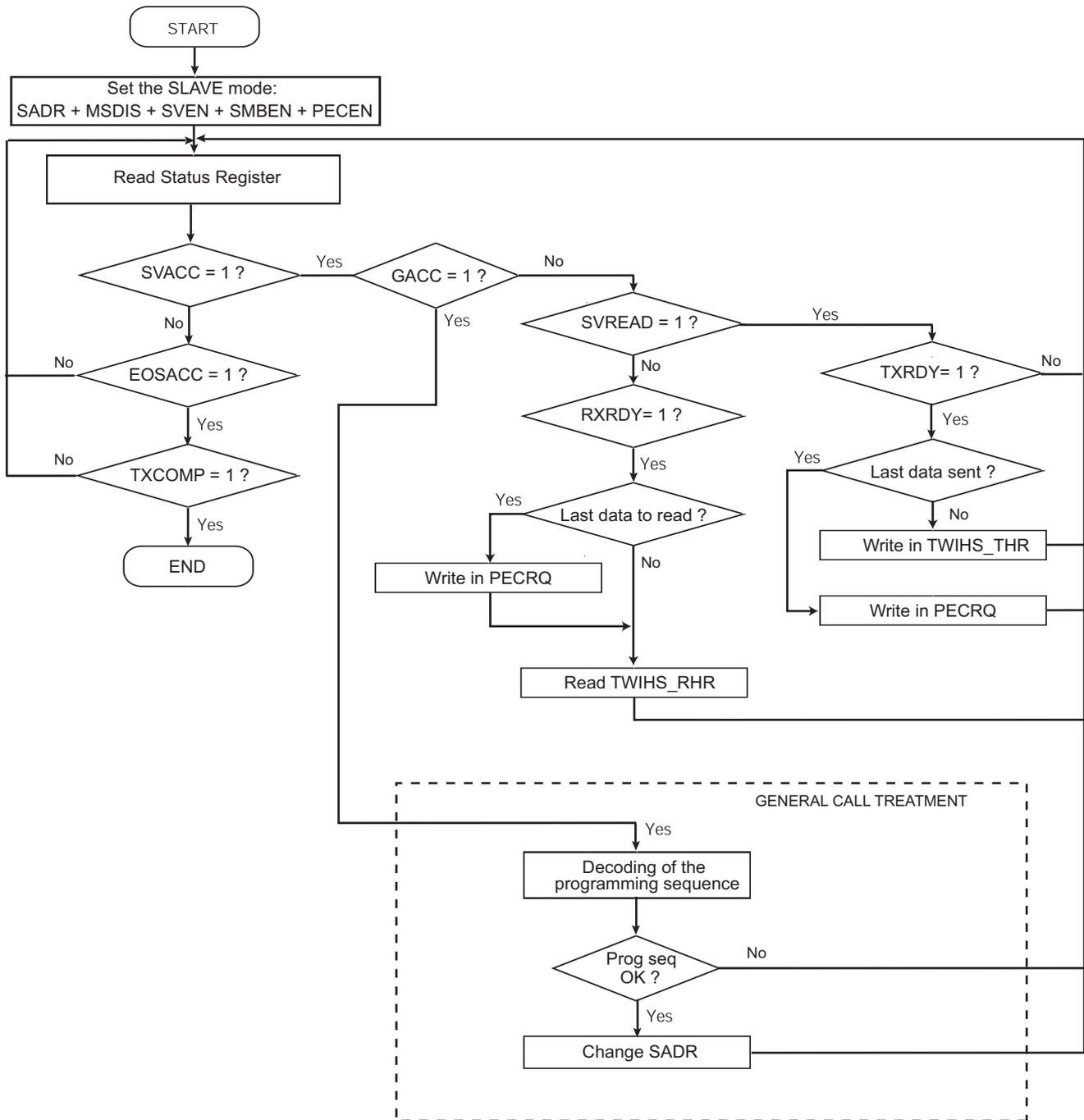
Figure 28-50. Read Write Flowchart in Slave Mode with SMBus PEC and Alternative Command Mode
