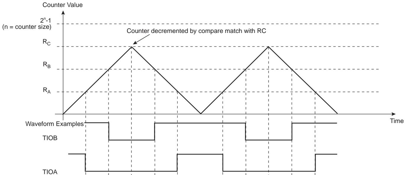
**Figure 34-15. WAVSEL = 11 with Trigger**
