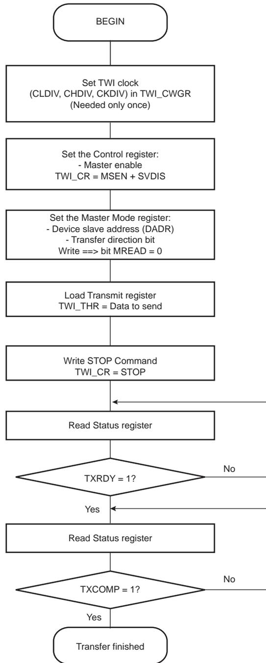
Figure 29-16. TWI Write Operation with Single Data Byte and Internal Address
