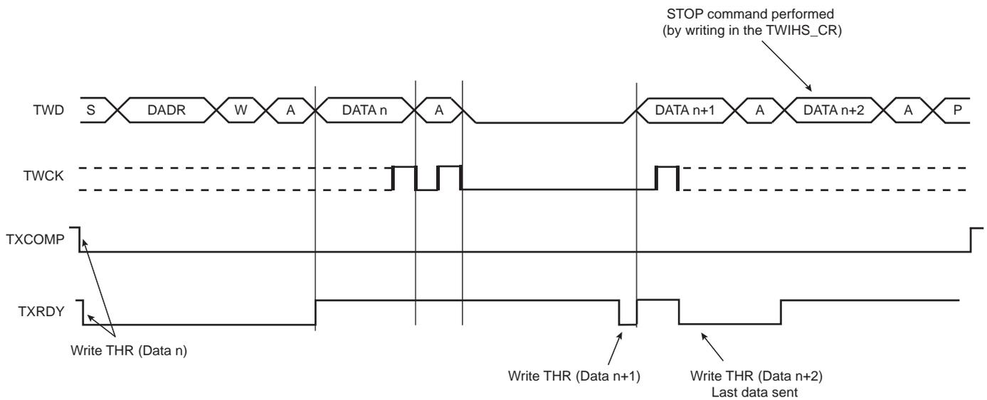
**Figure 28-9. Master Write with One Byte Internal Address and Multiple Data Bytes**
