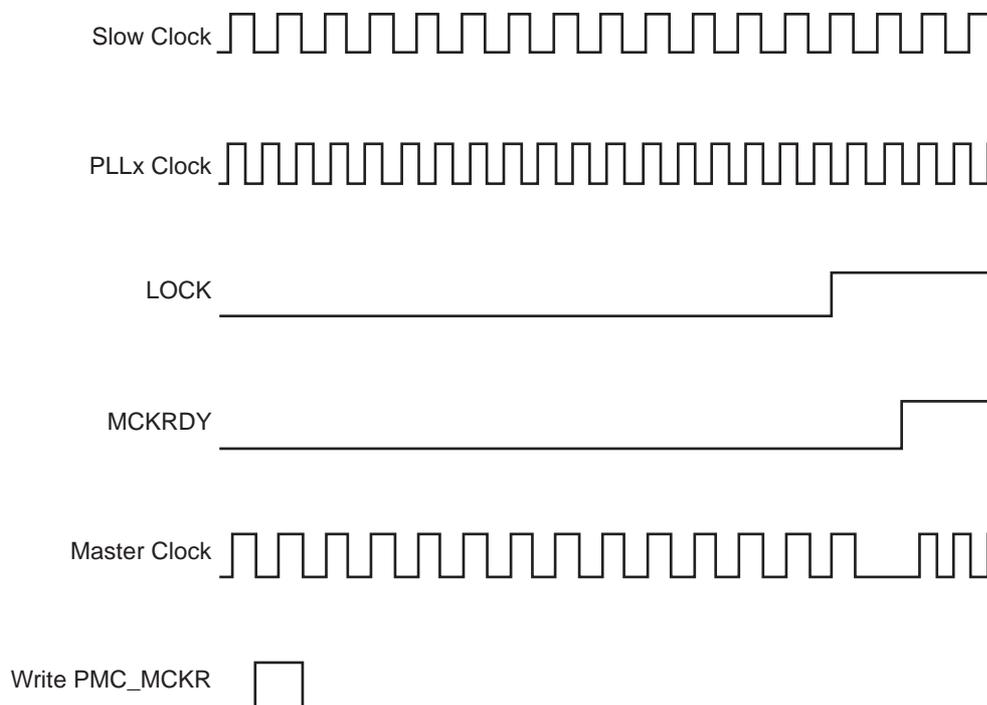
**Figure 24-8. Switch Master Clock from Main Clock to Slow Clock**
