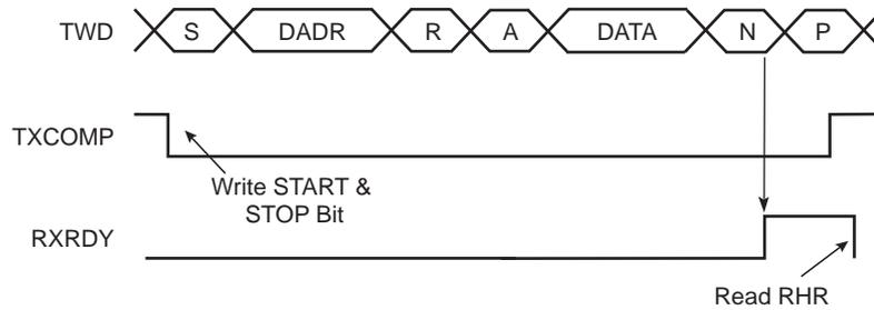
**Figure 28-11. Master Read with Multiple Data Bytes**
