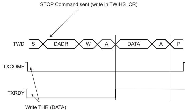
**Figure 28-8. Master Write with Multiple Data Bytes**
