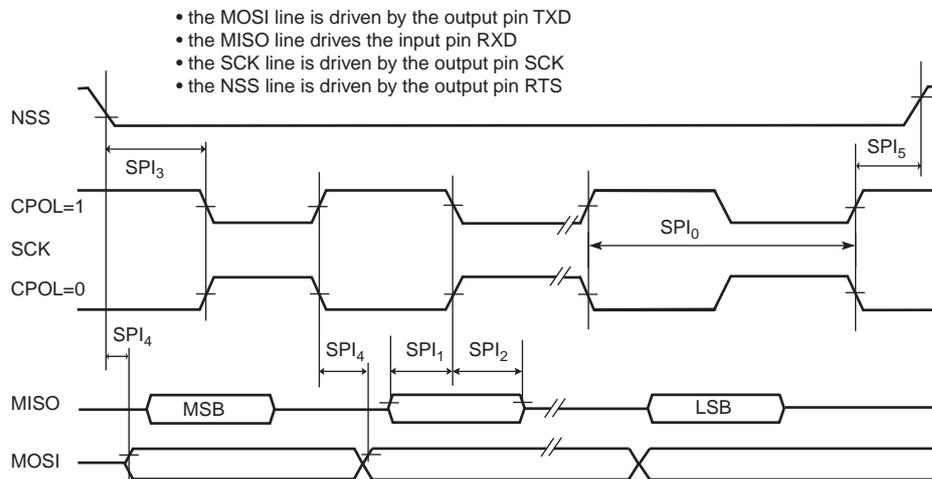
**Figure 36-16. USART SPI Slave Mode (Mode 1 or 2) r**
