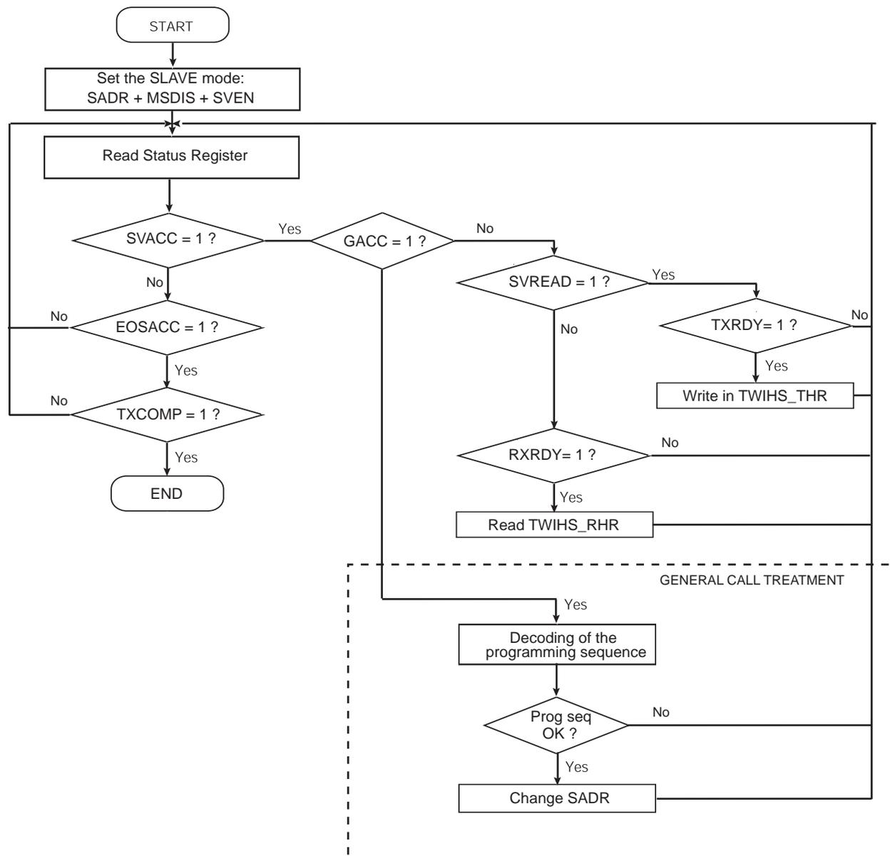
Figure 28-49. Read Write Flowchart in Slave Mode with SMBus PEC
