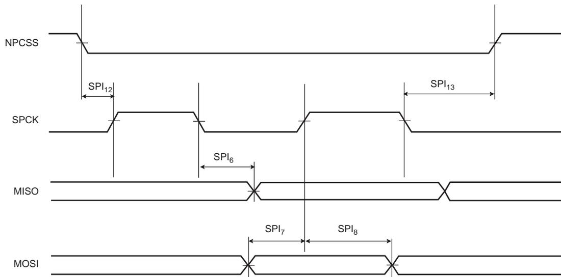
**Figure 36-14. SPI Slave Mode with(CPOL = NCPHA = 0) or (CPOL = NCPHA =1)**
