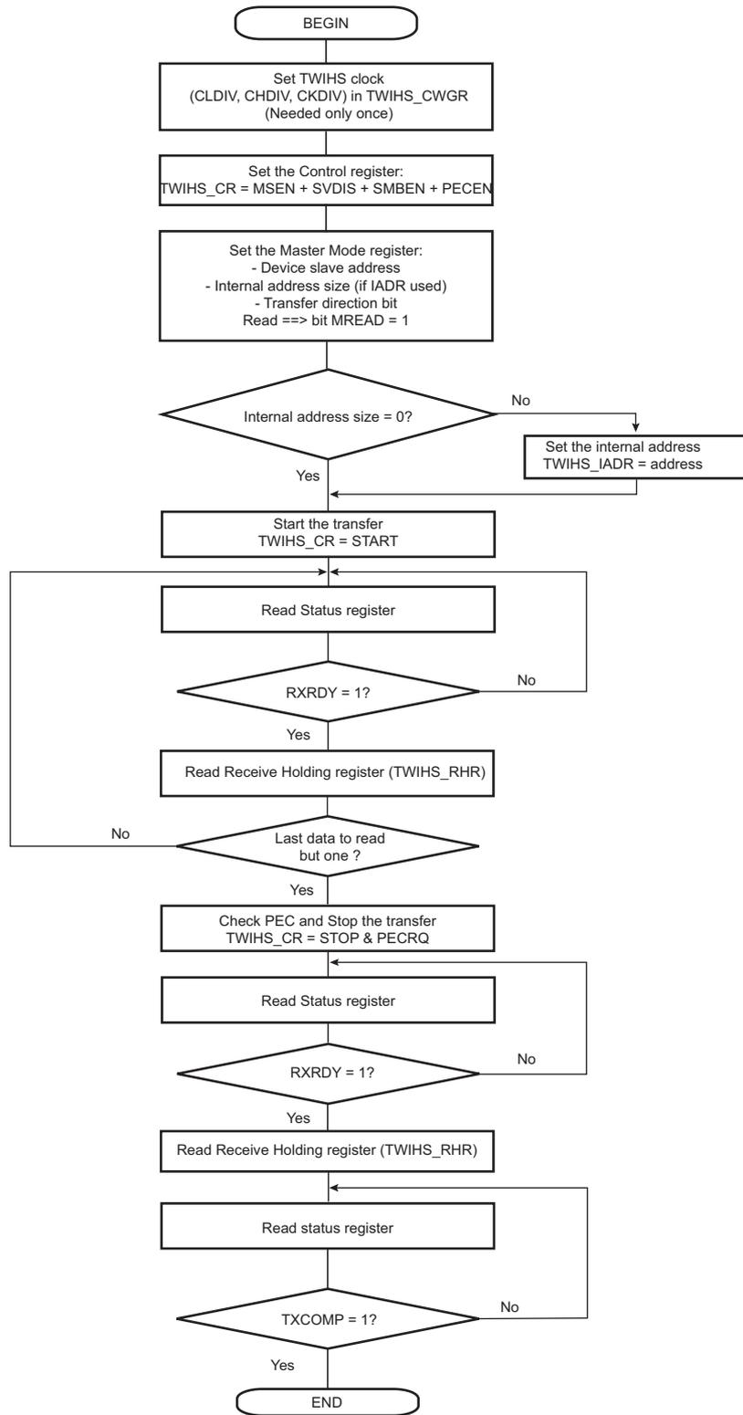
Figure 28-28. TWIHS Read Operation with Multiple Data Bytes with Alternative Command Mode with PEC
