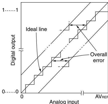
Figure 12-16. Quantization Error
