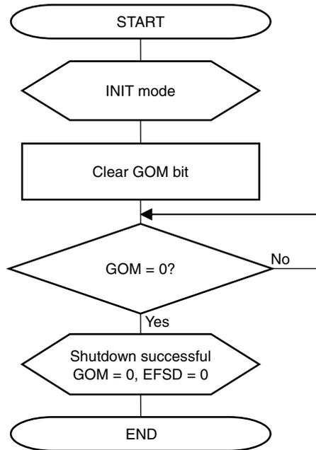
Figure 15-59. Forced Shutdown Process
