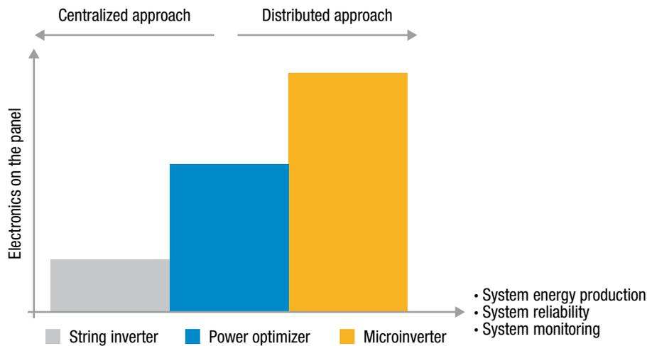
The following three photovoltaic grid-tied architectures are analyzed here:
