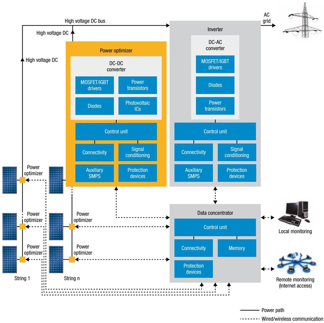
**Figure 4 High-voltage power optimizer based architecture (simplified block diagram)**
