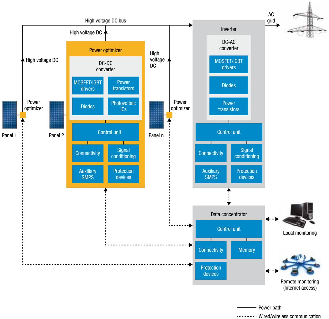
ST's product offering for power optimizer architecture is shown below. The key products for each functional block described above are described in the table below.
