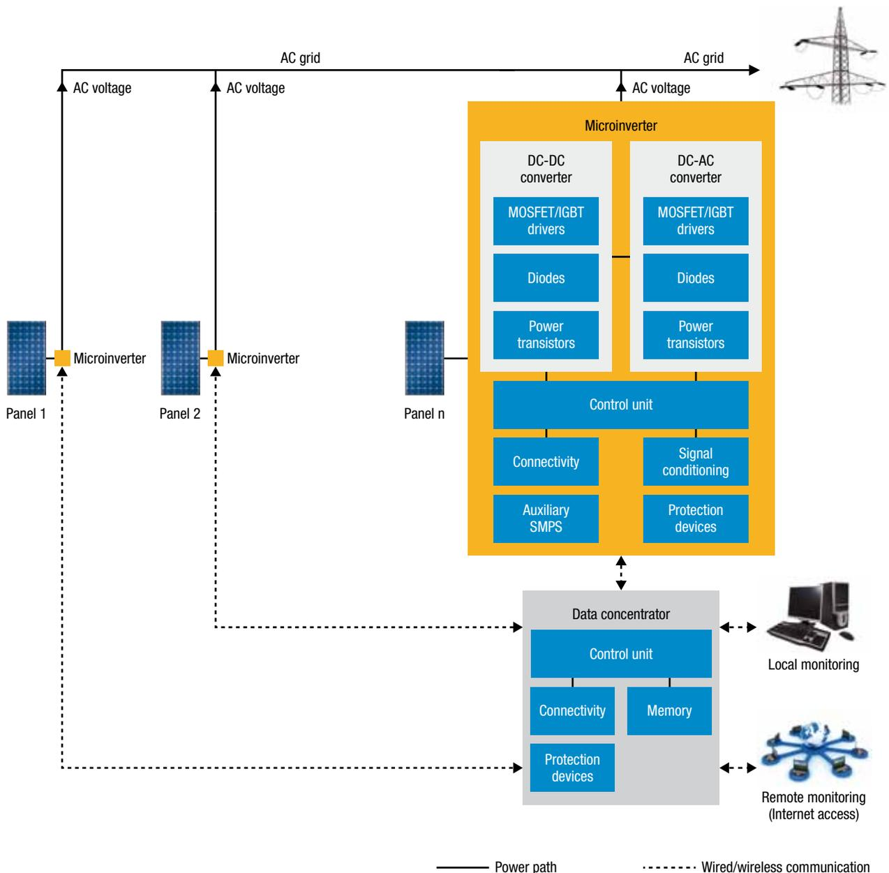
ST's product offering for microinverter architectures is shown below. The key products for each functional block described above are described in the table below.
