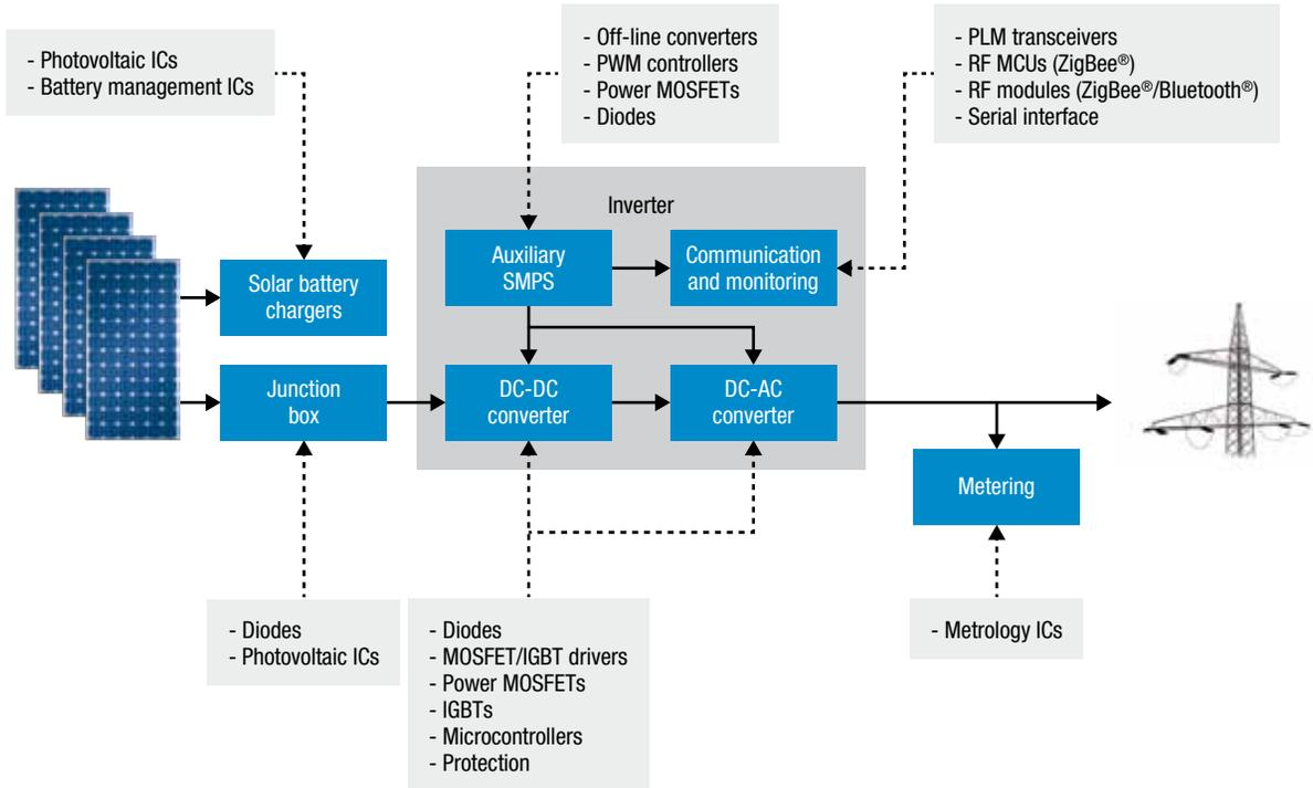
ST's innovative solar devices implement the MPPT (maximum power point tracking) algorithm to maximize the energy produced from each solar panel at any panel temperature and radiation condition and so to maximize the overall efficiency of the PV system.
