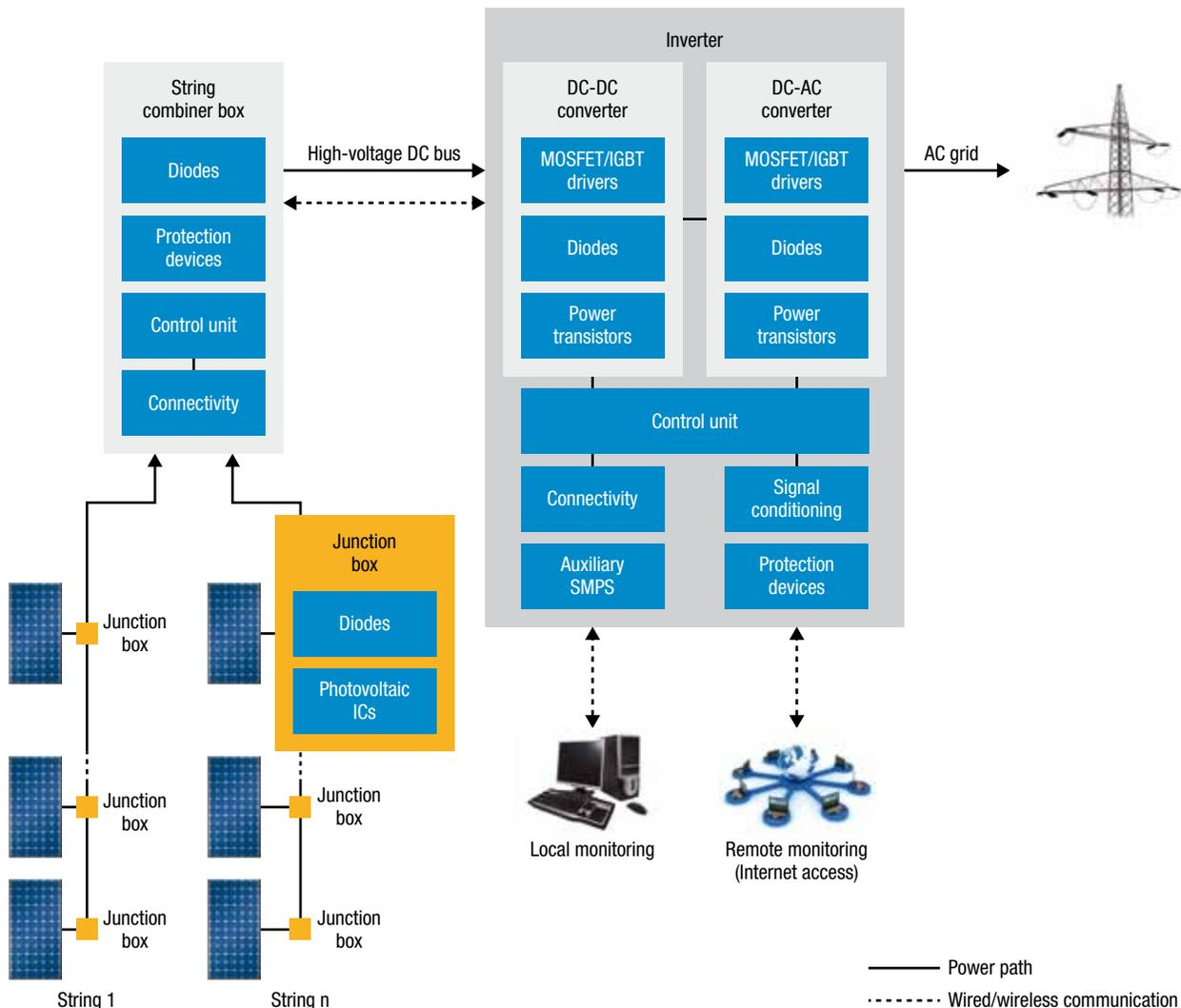
ST's product offering for the central inverter architecture is shown below. The key products for each functional block described above are described in the table below.
