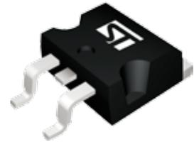
The package is RoHS compliant, uses green molding compound (bromine and antimony free), is lead-free, with 100% pure tin plating, withstands 260 °C IR reflow soldering and meets moisture sensitivity level 1 (MSL).
