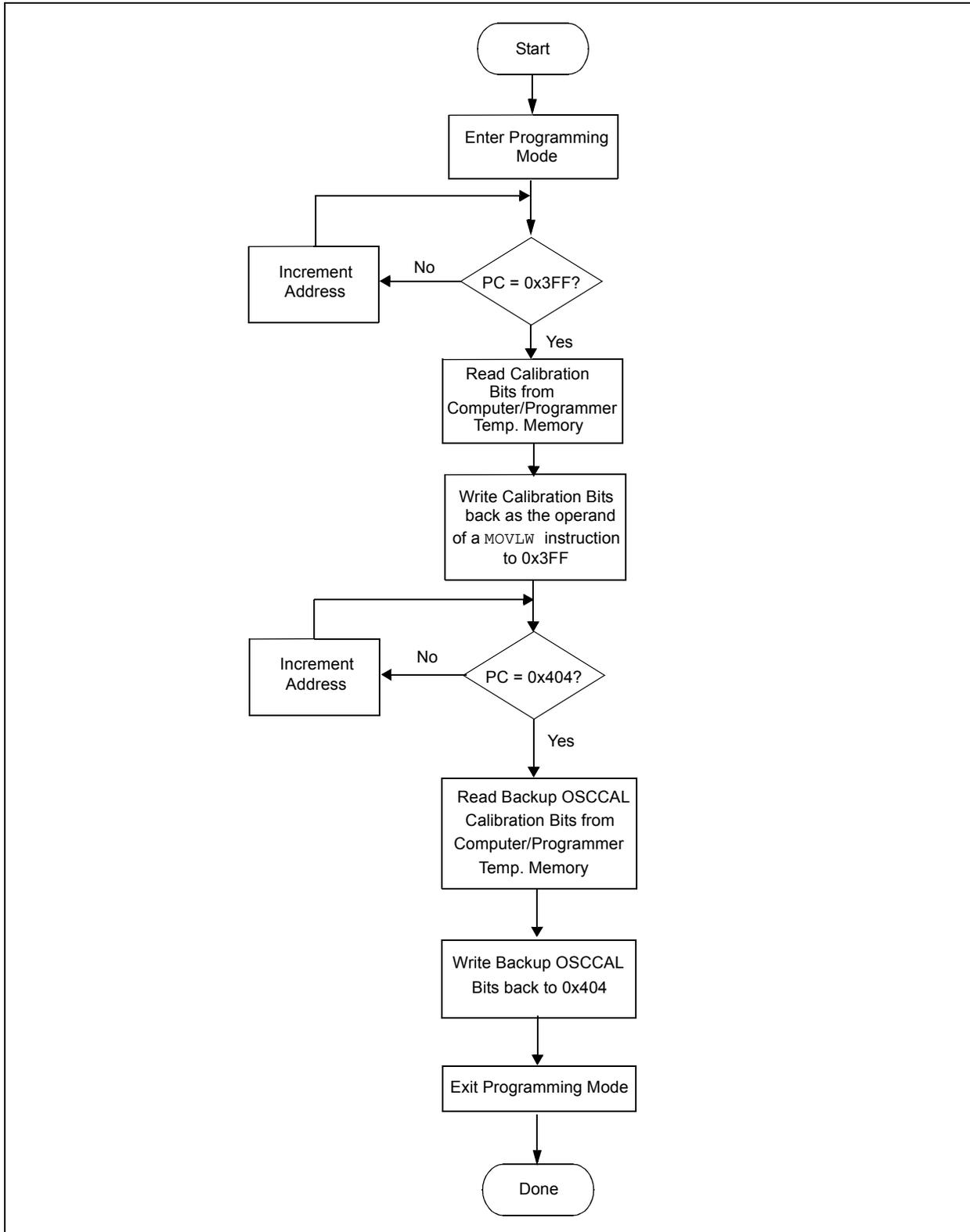
**FIGURE 3-10: PROGRAM FLOWCHART – PIC16F506 PROGRAM MEMORY**
