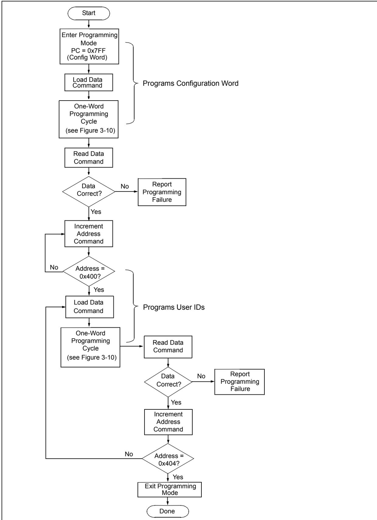
FIGURE 3-12: PROGRAM FLOWCHART – ERASE PROGRAM MEMORY, CONFIGURATION WORD
