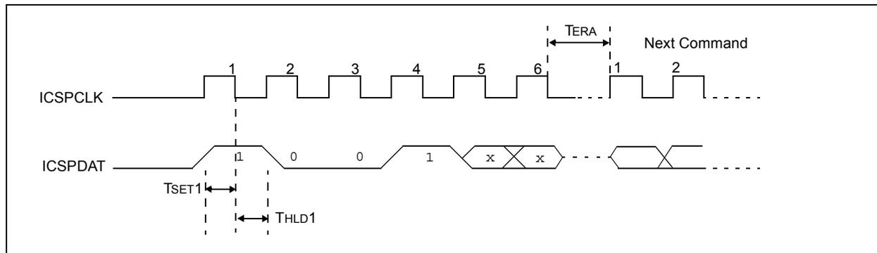
**FIGURE 3-8: READING AND TEMPORARY SAVING OF THE OSCCAL CALIBRATION BITS**
